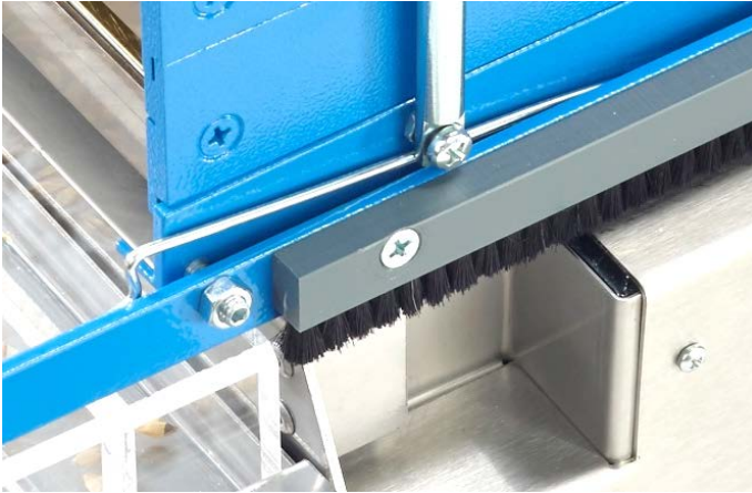
Figure 4: Correct installation position of the safety spring below the holding screw of the sieve stack
