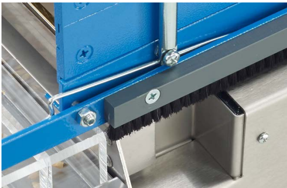
Figure 1: Position of safety spring during operation
