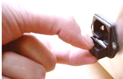
Figure 15: Renewal of the internal fuse
